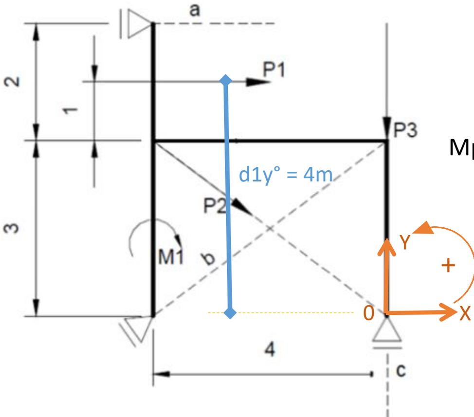
$$M_{p1}^{\circ} = P_1 \cdot d^{\circ} = -P_{1x} \cdot d_{1y}^{\circ} + P_{1y} \cdot d_{1x}^{\circ} = -10\text{KN} \cdot 4\text{m} + 0\text{KNm} = -40\text{KNm}$$
